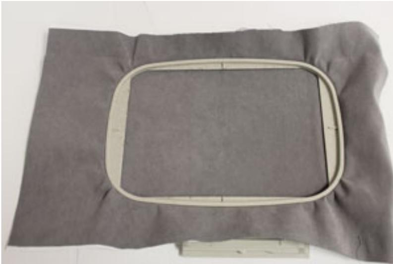
*Hoop the fabric with the stabilizer, and use temporary spray adhesive between the fabric and stabilizer for best results.*
