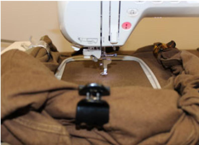
*Roll the excess fabric up to the sides of the hoop, and secure with clips.*
